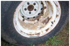
Original, non-floating, 5-lug axle with aftermarket dual wheels. Needs replacement. Note the absence of bolts around the center hub.
