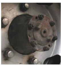
Close-up of center hub showing end-cap bolts on 6-lug axle.
